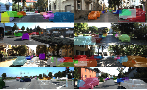
Fig. 22: Amodal instance segmentation results from ImageNet weights using RGB and occlusion edge refinement.
