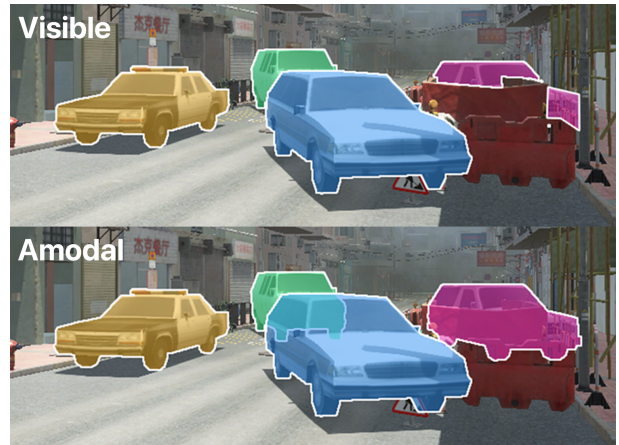
Fig. 1: Amodal instance segmentation segments the entire object while modal (visible) instance segmentation only segments visible regions
