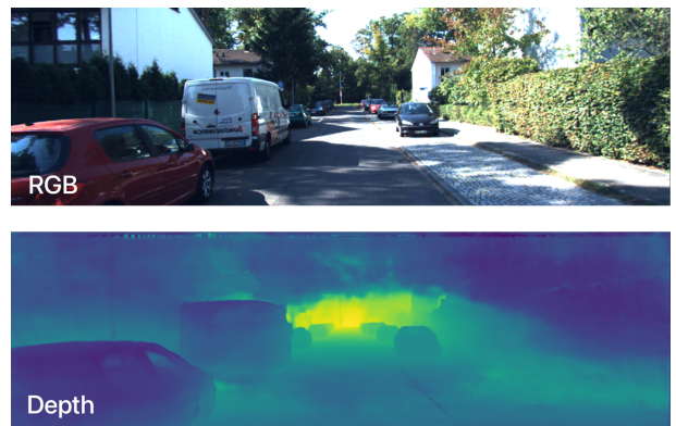
Fig. 9: Monocular depth prediction from a single RGB image from the KITTI dataset, the model used the BTS Network with a DenseNet161 backbone.
