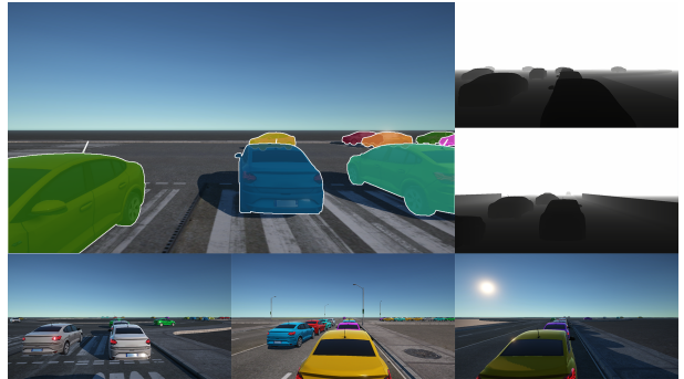
Fig. 6: The Openroads subset of RGSD, which contains RGB, depths and annotations of amodal and visible masks.
